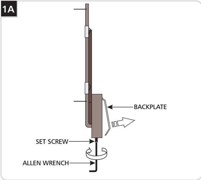
**1** Loosen (do not remove) the set screw at the bottom of the fixture and remove the backplate.
