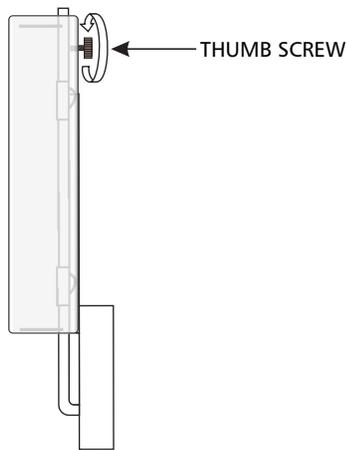
**NOTE:** Do not over tighten the thumb screw. Over-tightening may break the glass and cause injury.
