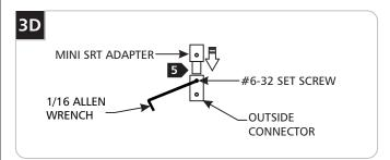
Install the Mini SRT adapter onto one end of the outside connector and tighten the #6-32 set screw with the 1/16 Allen wrench.
