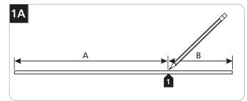
From one end mark the section of the extender that needs to be shortened (B), refer to the chart below for measurements.
