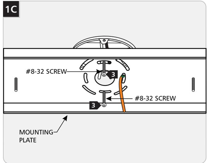
**3** Secure the mounting plate to the electrical box with the two #8-32 screws provided.
