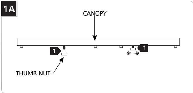
**1** Separate the mounting plate from the canopy by first unscrewing and removing the two thumb nuts.
