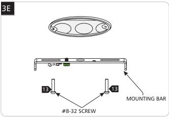
Secure the mounting plate to the junction box with #8-32 screws.
