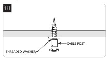
10 Tightly screw the cable post back onto the threaded washer.
