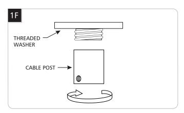
8 Unscrew the threaded washer to separate it from the cable post.
