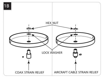
3 Use the lock washer and hex nut to attach either the coax only strain relief if using two cable supports or the aircraft cable strain relief, depending on the desired fixture configuration.
