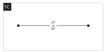
Mark the cable post location point at 47" or 93" away from the center of the junction box if using one post. Mark both locations for two posts.
