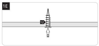
7 Screw the anchor in the rest of the way with a Phillips screwdriver.
