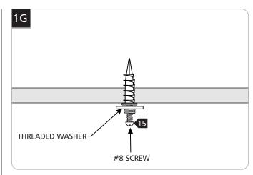
9 Screw the threaded washer onto the anchor with the long #8 screw.
