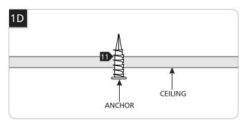
Tap the anchor at the marked point into the wall up to the threaded portion with a hammer.
