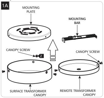
Remove the screws from the canopy to remove the mounting plate/bar. (Three screws for the surface mount and two for the remote.)
