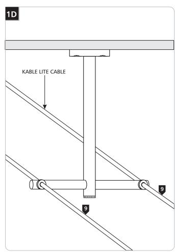
9 Run the Kable Lite cables coming from the turnbuckles through the bushings on the separation bar for all standoffs used in the run.
