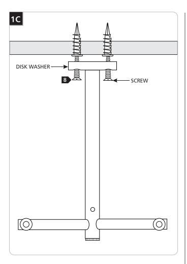
8 Secure the standoff by screwing the disk washer to the anchor with the provided two #8 screws.
