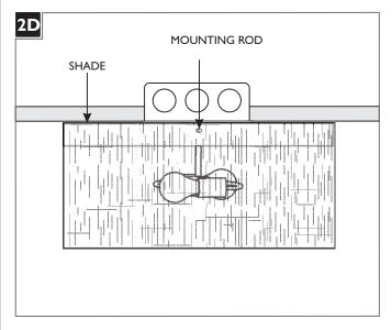
Align the shade with the fixture base and re-install the three mounting rods by hand.
