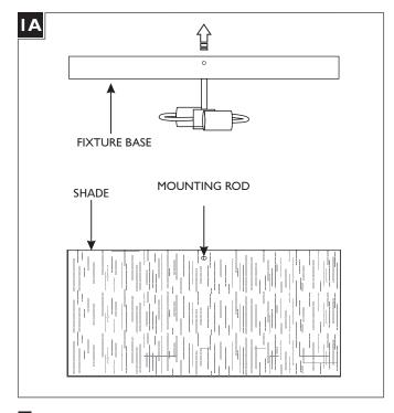
Remove the three mounting rods by hand and separate the shade from the fixture.
