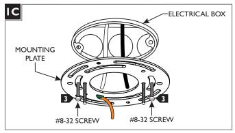
Mount the mounting plate to the electrical box with the two #8-32 screws.
