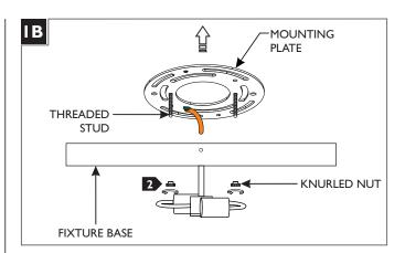
2 Remove the mounting plate from the fixture by unscrewing the two knurled nuts from the two threaded studs.
