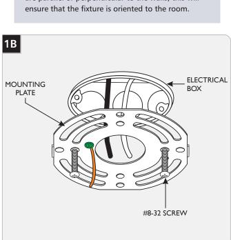
Mount the mounting plate to the electrical box using the provided #8-32 screws.
