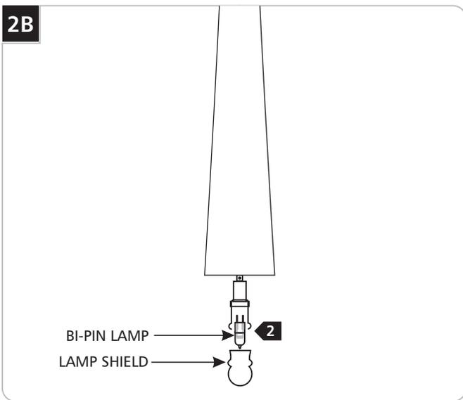
**2** Remove the lamp shield and the old lamp.
