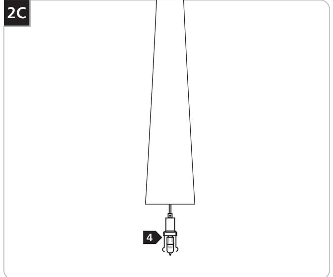
**3** Handle the new replacement lamp with a soft cloth to prevent the natural oils on the fingertips from collecting on the lamp. This will help extend the life of the lamp.
