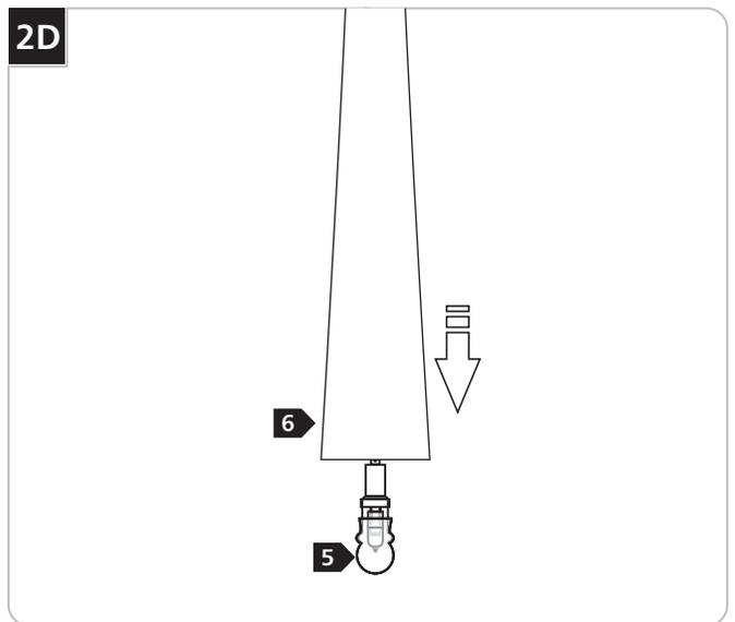
**5** Push the lamp shield onto the spring clip.
