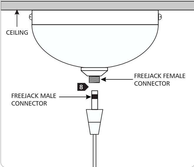
**8** Screw the fixture FreeJack male connector into the FreeJack female connector.
