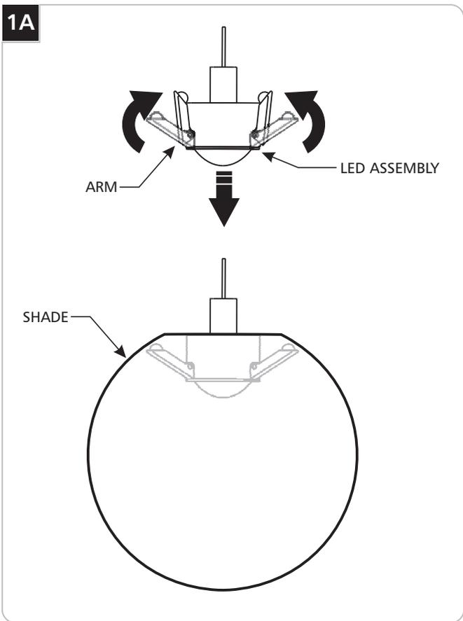
**1** Fold and hold the arms, insert the LED assembly into the shade, center the LED assembly to the shade and release the arms. Adjust as necessary.
