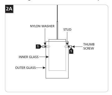
1 Line up the outer glass holes with the inner glass studs and secure the outer glass to inner glass with provided thumb screws and nylon washers.
