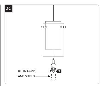
3 Remove the lamp shield and the old lamp.
