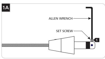
Back out (do not remove) the set screw on tip of the connector with the provided Allen wrench.
