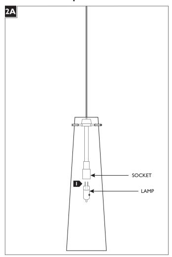
**NOTE:** To reduce the risk of a burn or electric shock during relamping, disconnect the power to the fixture.
